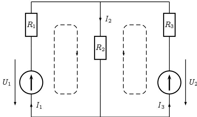
$$-U_1 + R_1 I_1 + R_2 I_2 = 0 \quad (1)$$
