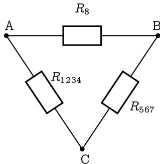
$$R_{AB} = \frac{1}{\frac{1}{R_8} + \frac{1}{R_{1234}+R_{567}}} \approx 44,385\Omega$$
