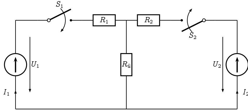
$$l = 2000m \quad \rho = 1,78 \cdot 10^{-2} \frac{\Omega \text{ mm}^2}{m} \quad A = 1mm^2$$
