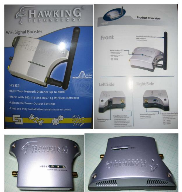
The device is supplied with a AC-DC power supply. The power supply provides 12V 1.5A to the Booster. I measured an averaged current consumption of 80mA in receive/standby mode and 200 mA in active mode (during a file transfer in 802.11g mode). Please note that WLAN is a TDD/TDMA system which means it uses
