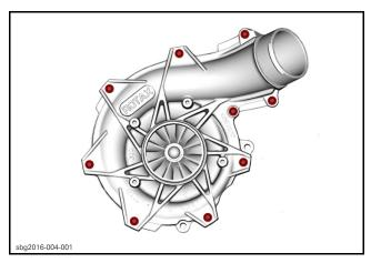
4. With locking tool in place, remove cup nut and shim holding impeller, discard cup nut only.
