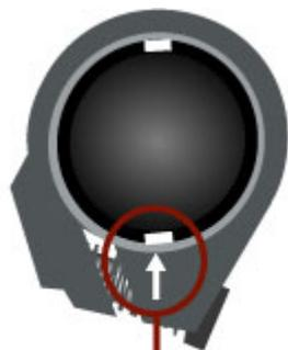
Arrow on clamp and slot in frame need to be aligned
